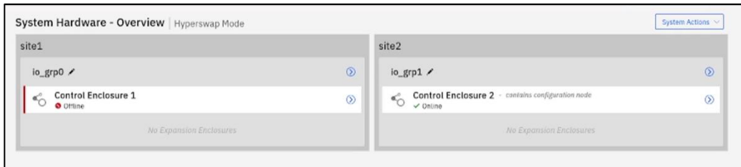
Figure 9: IBM FlashSystem on Site 1 is off
